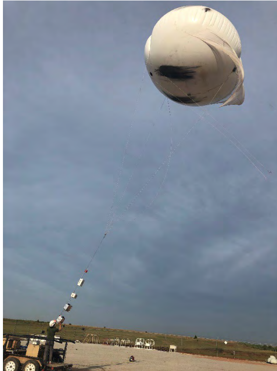
Figure 3. ARM's tethered balloon systems can go into and above clouds to collect data related to horizontal wind, ice microphysics, turbulence, thermodynamic state, aerosols, and the cloud-top environment.
