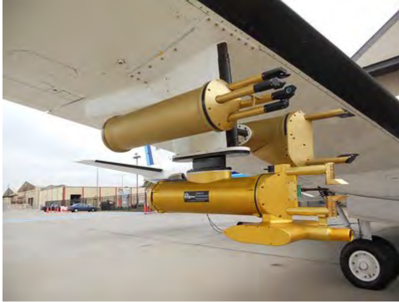
Figure 6. Instruments mounted under G-1 wing.
