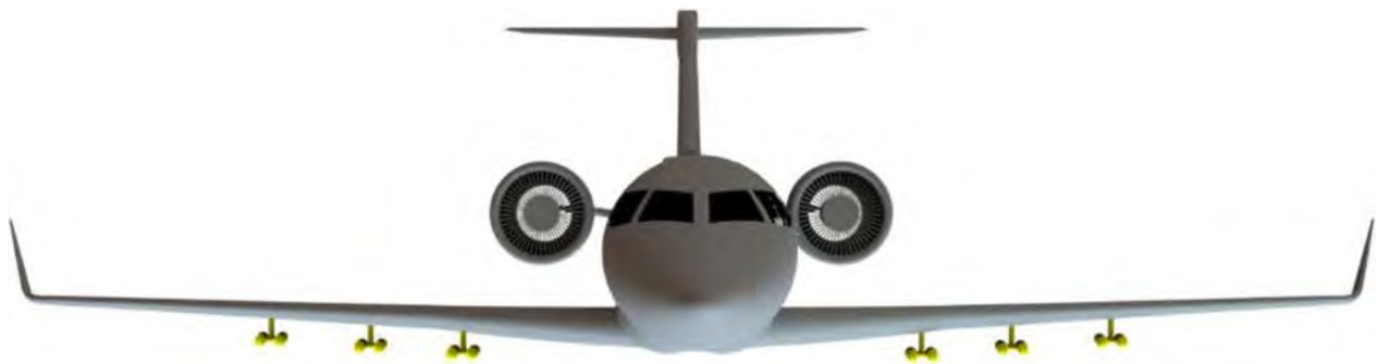
Figure 7. A notional installation for the wing pylons.
